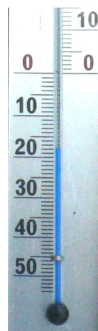
Fig. 1. Thermometer based on liquid thermal expansion.
