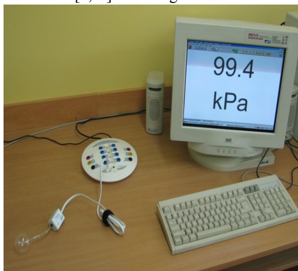
Fig. 3. Measuring arrangement based on Coach system
