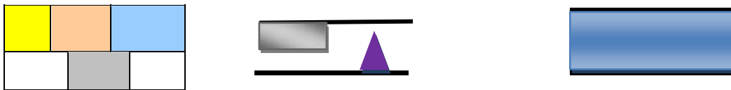
Figure 1. The scheme of dielectric materials filling flat capacitors
